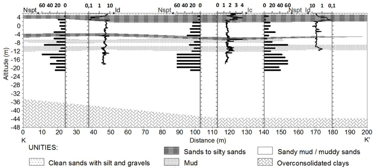
Fig. 3. Litostratigraphic cross section K-K' at Aveiro site.
