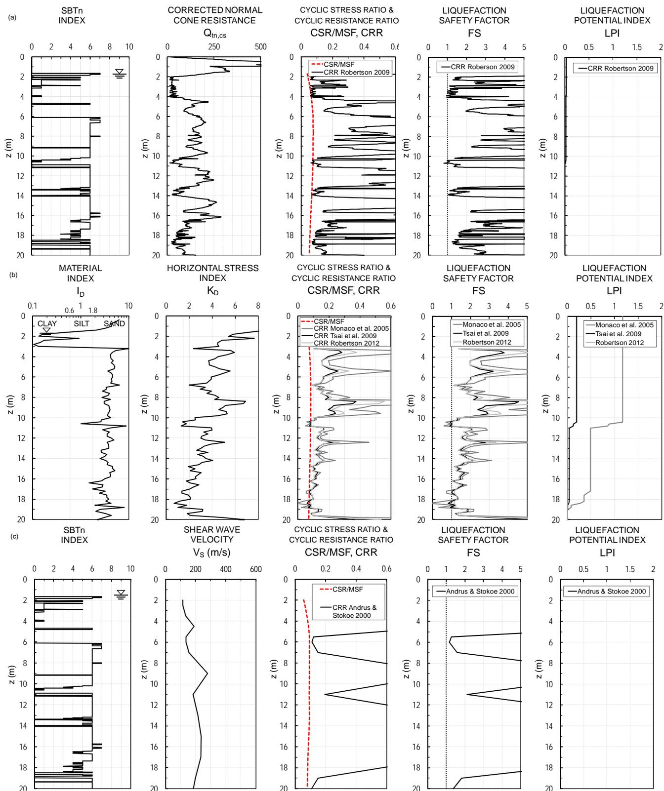
Fig. 4. *LPI* estimations from CPTu (a), DMT (b), and  $V_S$  measurements (c) for SCPTu2-1B and DMT4-1B tests, considering the Seismic Action 1 at Aveiro test site.
