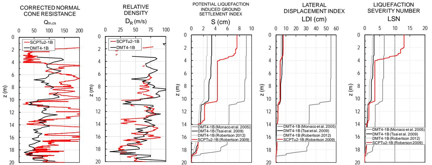
Fig. 5.  $S$ ,  $LDI$  and  $LSN$  estimations for SCPTu2-1B and DMT4-1B, considering the Seismic Action 1 at Aveiro test site.
