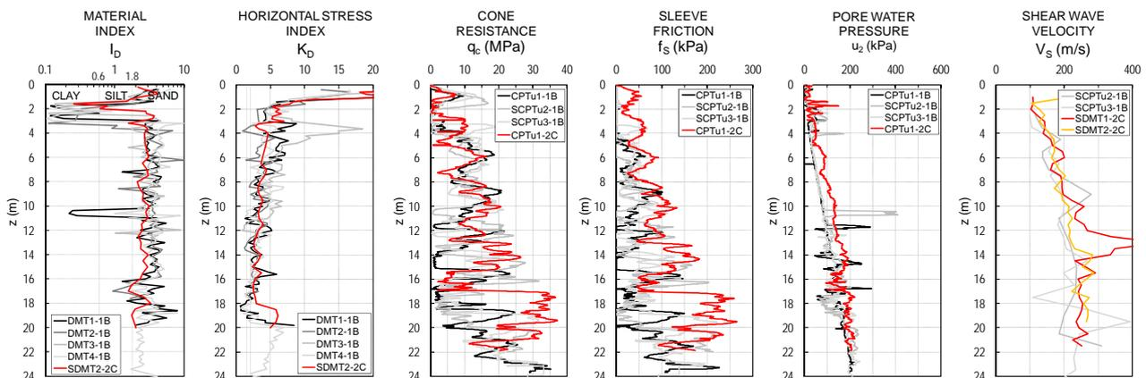
Fig. 2. DMT/SDMT and CPTu/SCPTu results for two site investigation campaigns (phase 1B, phase 2C).
